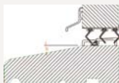
Standard 140mm Hardwood Sill with Mobility Threshold*
